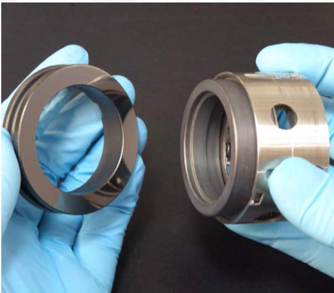
*Mechanical pump seal with diamond faces*
