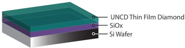
Standard silicon wafers with a thermal SiO<sub>2</sub> layer (nominal 1 micron thickness) followed by UNCD Aqua 25, 50, or 100. These substrates are ready for further MEMS processing using standard surface micromachining techniques to make UNCD-based cantilevers, resonators, diaphragms, and diamond windows. UNCD DOI Wafers are offered for all of the family of UNCD materials. Wafer sizes available are 100, 150, 200, and 300 mm.
