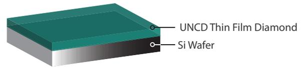
A prime silicon wafer with a thin film of UNCD. DoSi Wafers are offered for all of the family of UNCD materials. Wafer sizes available are 100, 150, 200, and 300 mm.
