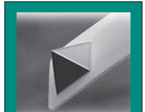
UNCD AFM probe made from DCI Wafer
