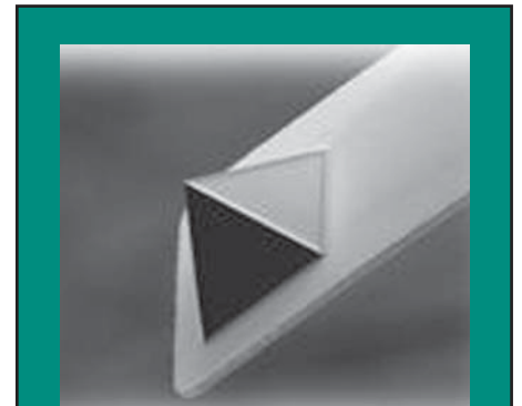
UNCD AFM probe made from DCI Wafer
